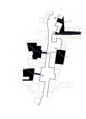
Yards channel water run-off.
